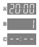
When both auto channel set and auto clock set have been completed successfully the correct current time will be displayed after the **OK** button is pressed in item **3** on page 6.
